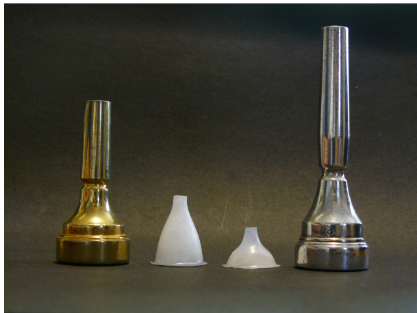
Figure 7: The two mouthpieces tested, together with wax castings of the cup shapes. The flugelhorn mouthpiece is on the left, the trumpet mouthpiece on the right.
