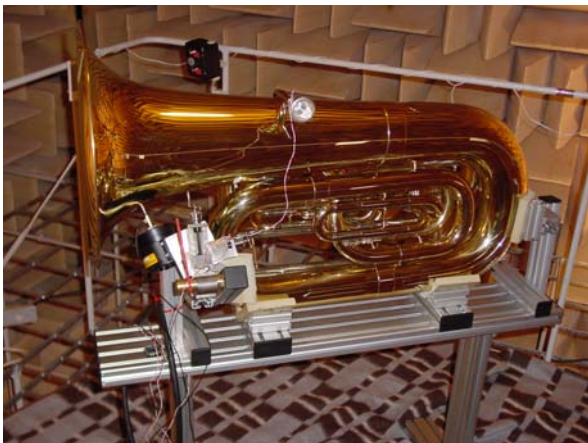
Figure 5: Arrangement to the simulation of the operating oscillations without airborne sound
