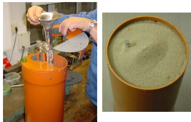
Figure 6: Sand back-filling of a trumpet
