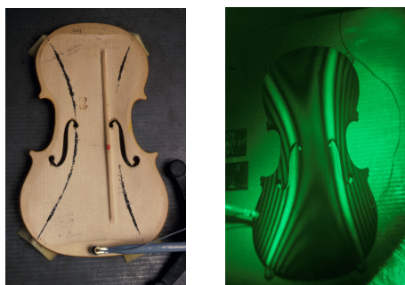
Figure 1: A Chladni pattern and interferogram of a mode of a free violin plate. Note the appearance of nodes in the two cases.
