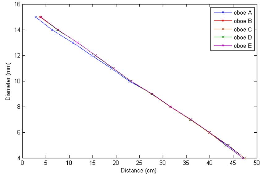
Differences in the impedance partially explained by discrepancies in the bore profiles.
